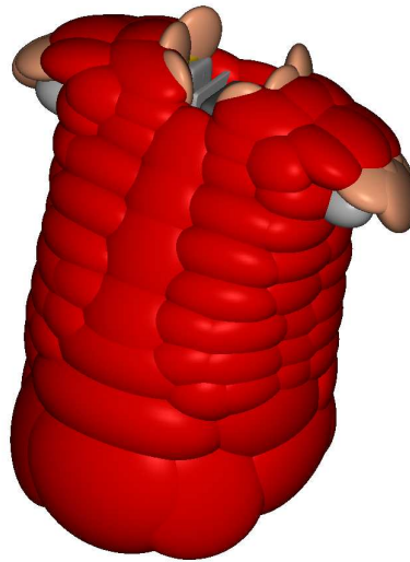
Figure 9.5: THOR-50M ellipsoid thorax
