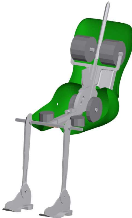
Figure 34.1: The MADYMO H-point manikin model.
