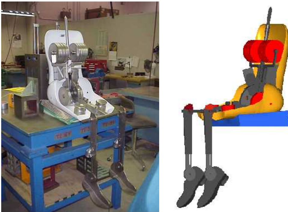
Figure 34.2: The experimental set-up of the H-point measurement of a block foam (left) and the numerical simulation of the experiments with the H-point manikin model (right).
