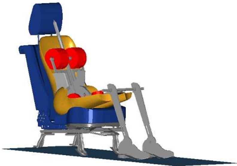
Figure 34.3: The H-point manikin model in a real car seat.
